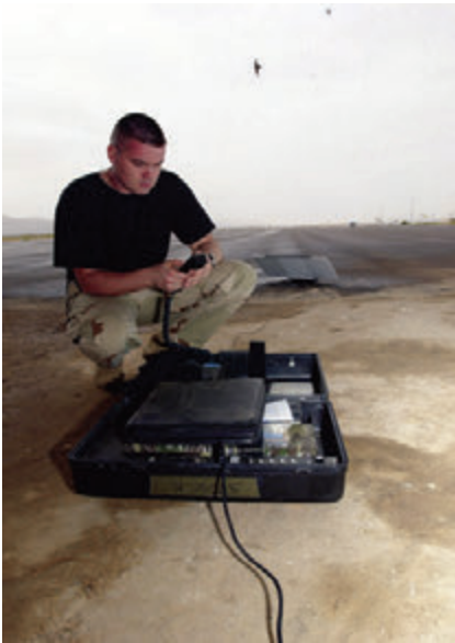
An INMARSAT mobile satellite communications device
