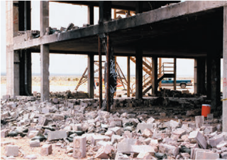
DTRA assesses the effects of various high explosive weapons through blast tests at its Albuquerque test site.
