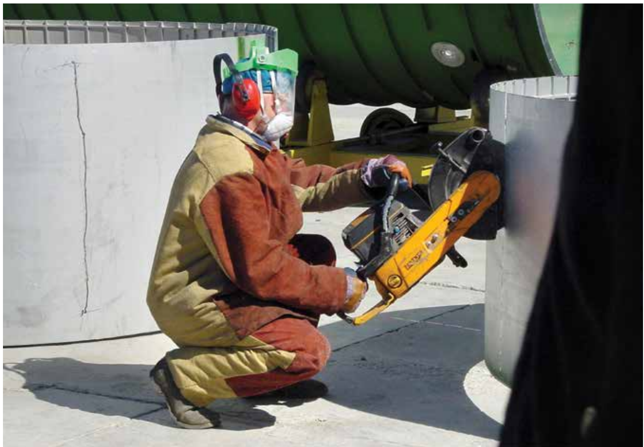
CTR provided power saw dismantling missiles
