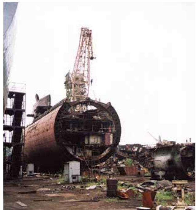
Dismantlement of Russian nuclear submarine
