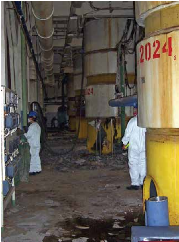
Fermentors inside the Stepnogorsk BW Production Complex
