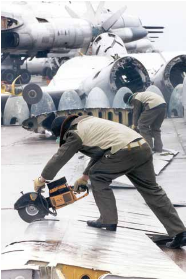
CTR equipment being used in heavy bomber elimination
