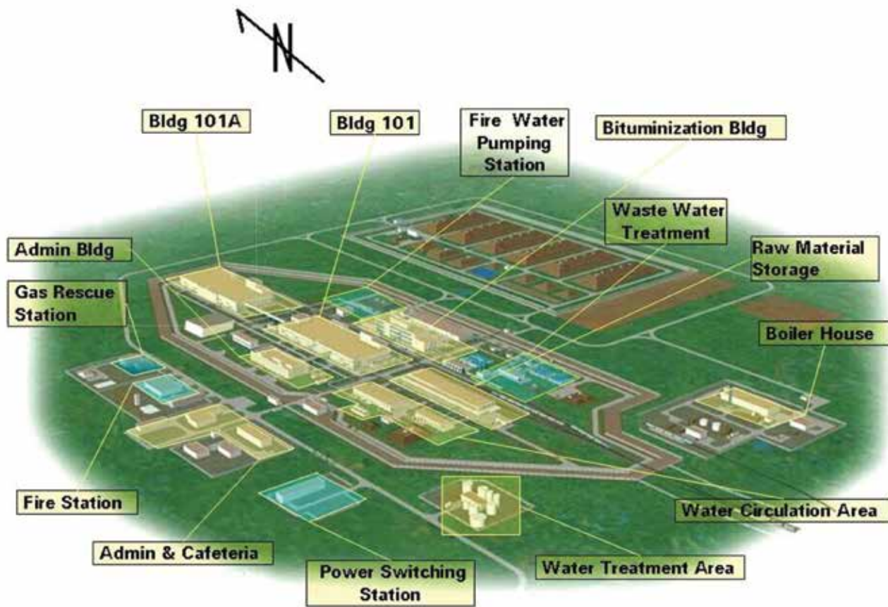
Schematic of Chemical Weapons Destruction Facility, Shchuch'ye
