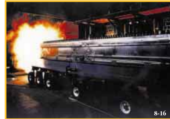
DNA EM rail gun being test fired.
