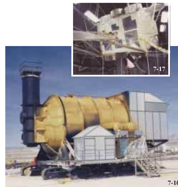
DoD satellite test chamber (HURON KING). INSET: Satellite suspended inside test chamber.
