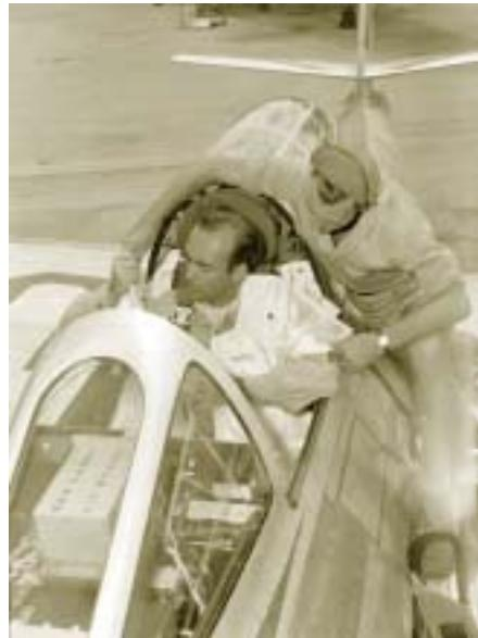
Protective lead-glass cloth shroud being placed on an Air Force pilot during sampling operations.
