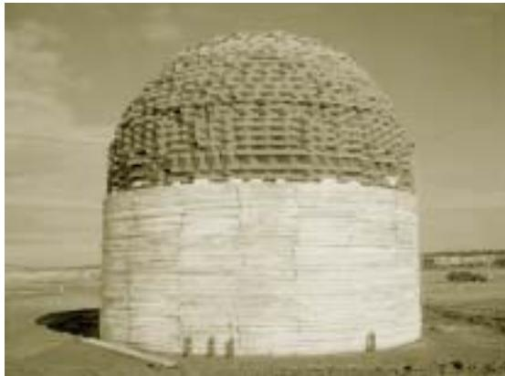
MIXED COMPANY: 500-ton TNT test stack, November 1972.
