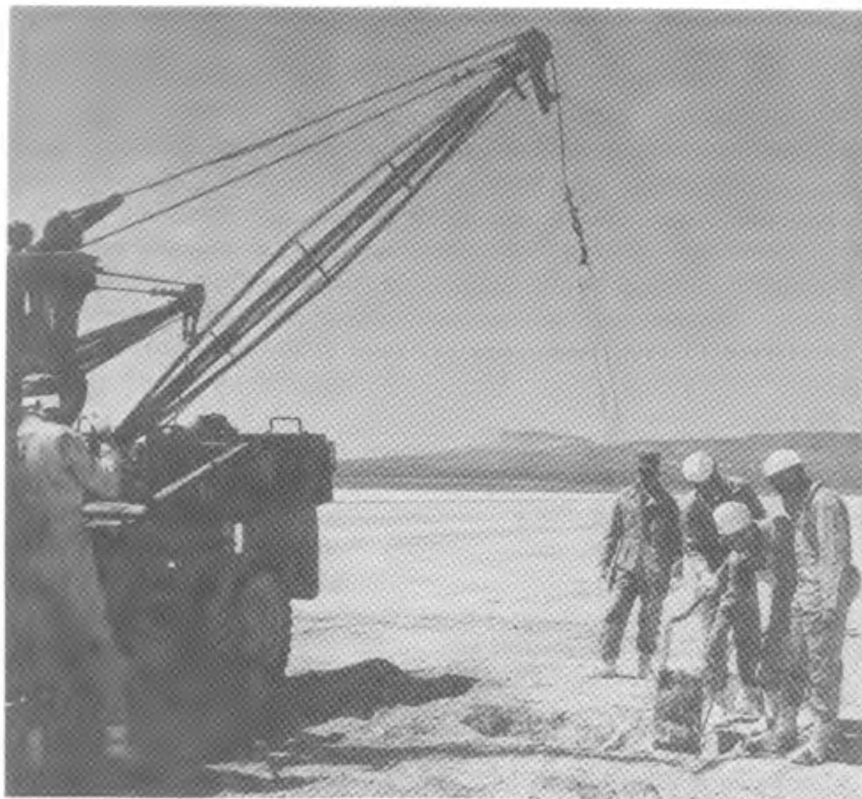
Figure 4-2: PROJECT 1.6 PERSONNEL REMOVE ACCELEROMETERS USED TO MEASURE GROUND SHOCK
