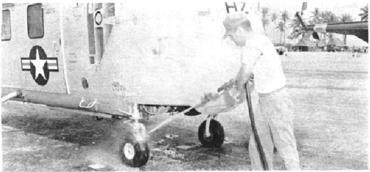
Figure 30. Removing radioactivity from a helicopter, REDWING.
