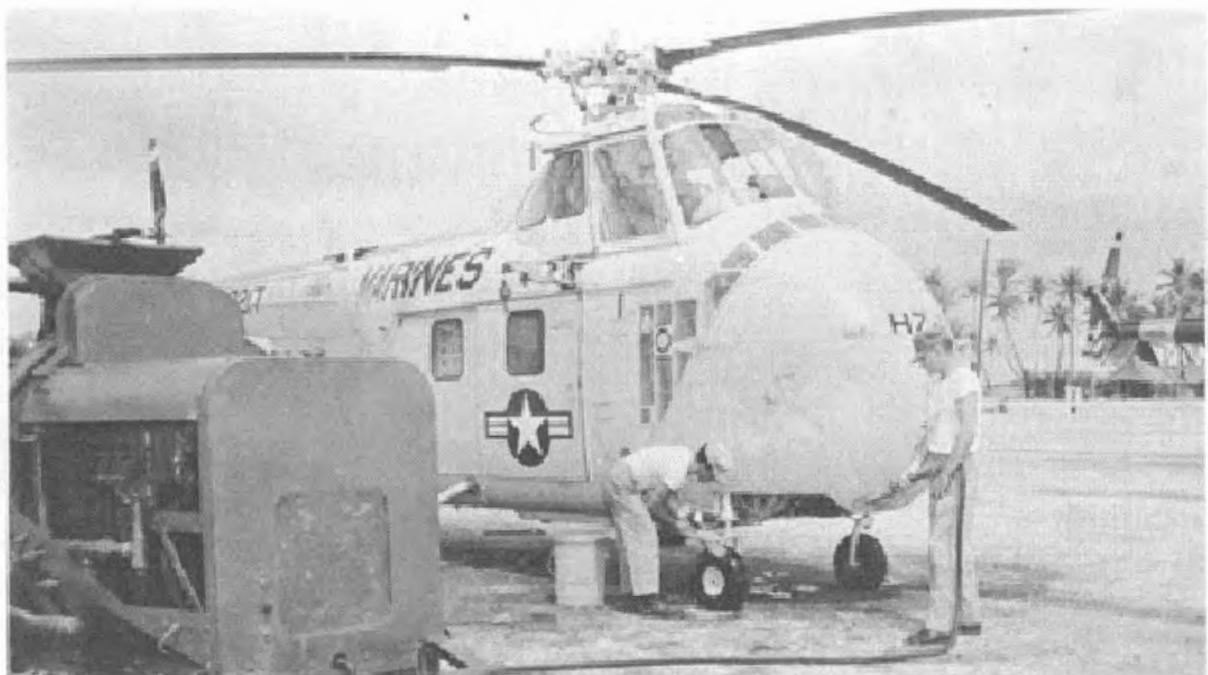
Figure 29. Scrubbing helicopter to remove contamination, REDWING.
