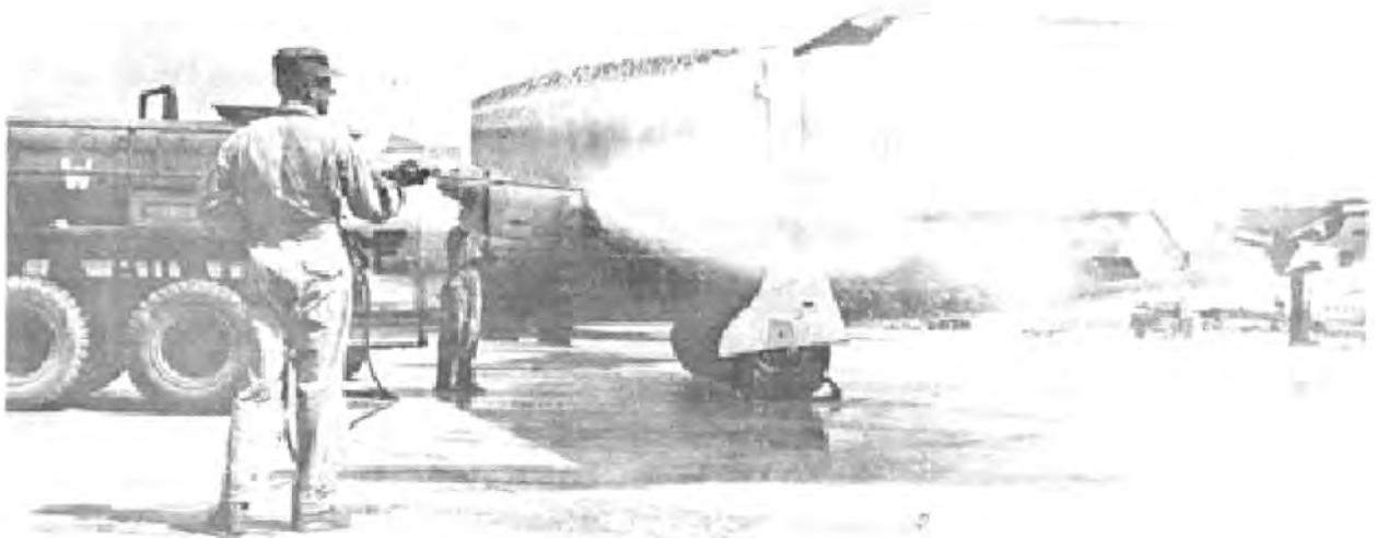
Figure 32. Decontaminating a B-57 sampler aircraft after flight through a nuclear cloud, REDWING.
