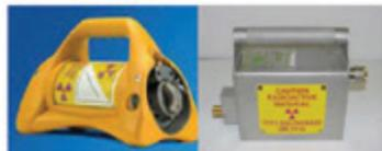
Iridium-192 Radiography Cameras with Depleted Uranium Shielding
