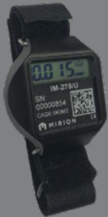
**Description:** Fielded as the IM-276PD (Navy) and the IM 278/U (Army), the dosimeter will provide a sensor to record and retrieve a Service member's radiation exposure from occupational to tactical levels.
