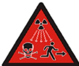
Dangerous Radiation Sources Symbol only on inside of device housing. If seen, device has been taken apart.
