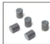
Uranium Reactor Fuel Pellets
