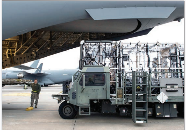
The Transport Isolation System or "TIS", a medical containment system, can be loaded onto a C-17 Globemaster III or a C-130 Hercules. (USAF photo)
