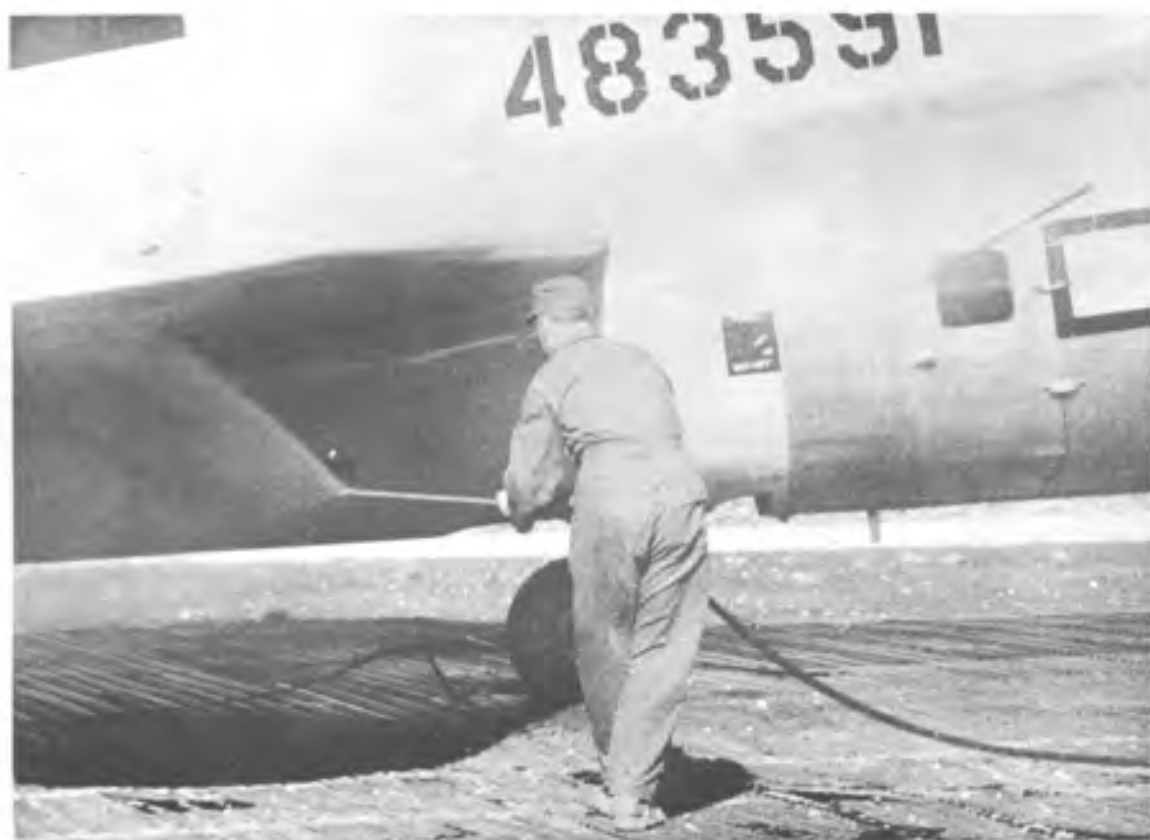
Figure 36. Decontamination of SANDSTONE B-17 drone sampler.
