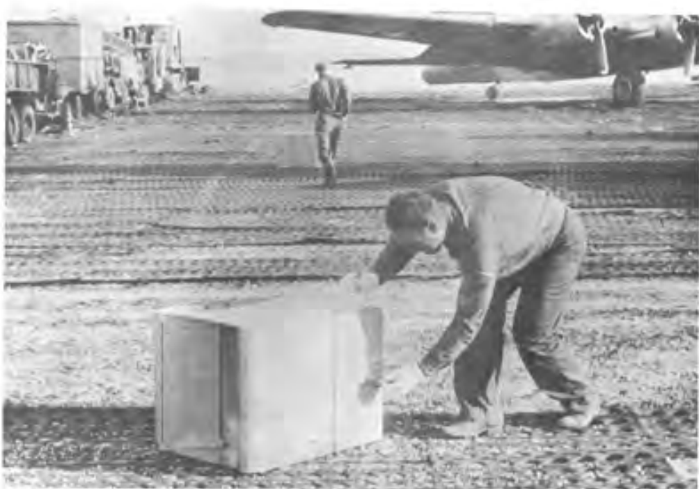
Figure 20. Man pulls lanyard to remove one of two filter-paper holders from top filter unit following shot ZEBRA, Operation SANDSTONE.
