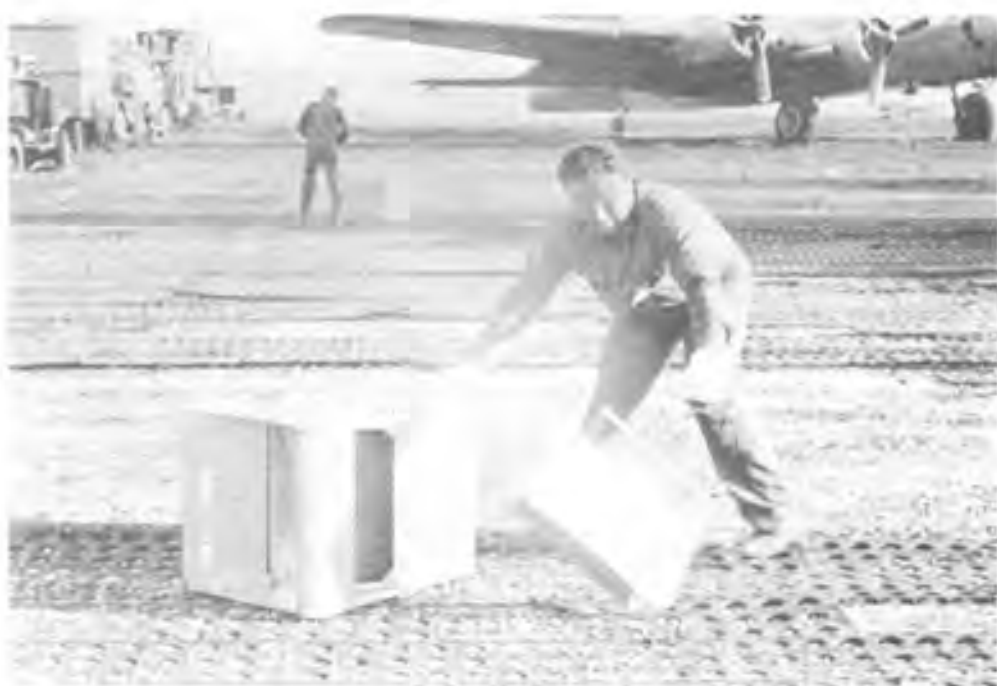
Figure 21. Lanyard pulls filter-paper holder free from top filter unit following shot ZEBRA, Operation SANDSTONE.
