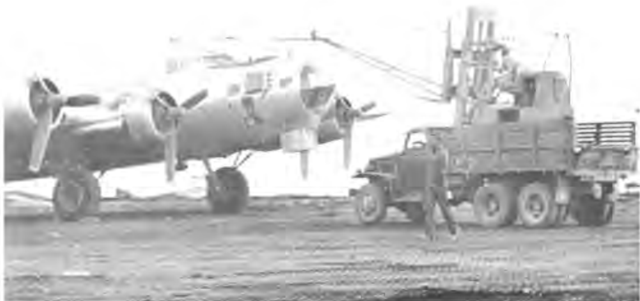
Figure 17. Drone B-17 at Enewetak after shot ZEBRA, Operation SANDSTONE, approached by truck with forklift with extension arm to grasp top sampler box. Lower sampler box is under nose.
