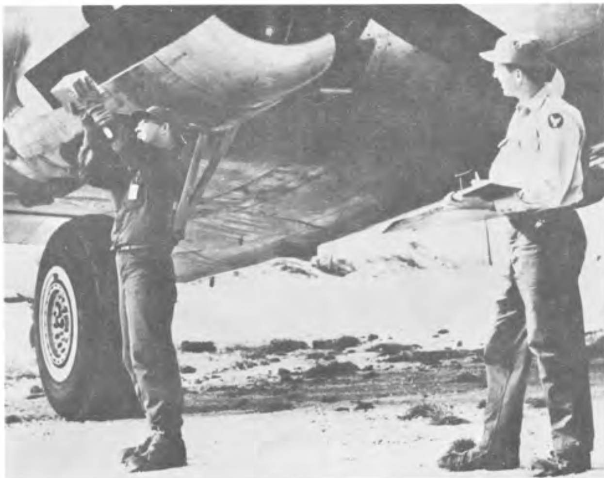
Figure 34. Monitors record radioactivity of SANDSTONE drone sampler before decontamination.
