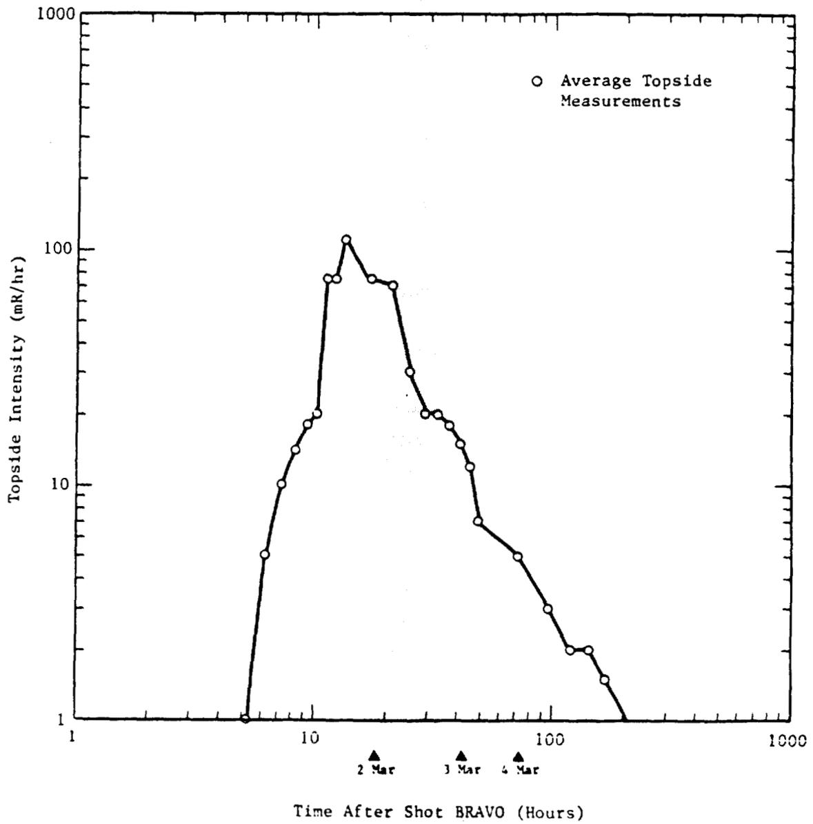
Figure 8. Topside intensity on USS COCOPA (ATF-101) following Shot BRAVO.
