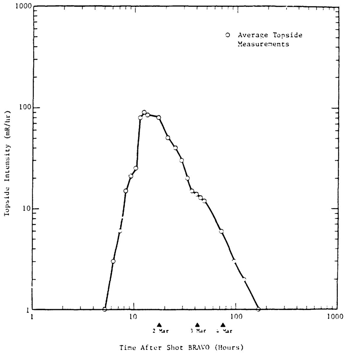
Figure 17. Topside intensity on USS PC-1546 following Shot BRAVO.
