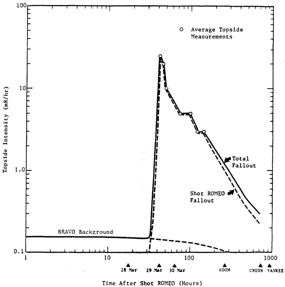
Figure 9. Topside intensity on USS COCOPA (ATF-101) following Shot ROMEO.
