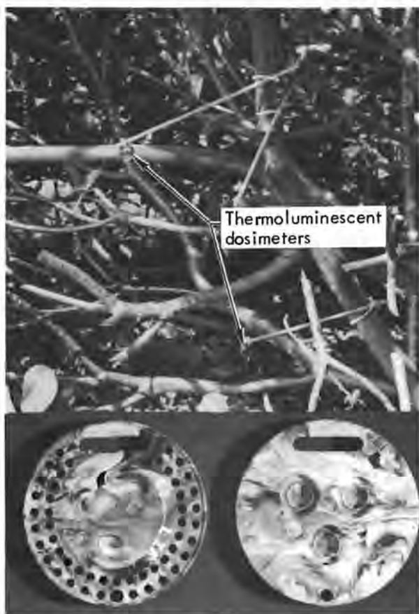
Fig. 38. Field placement of TLD's with enlarged view of TLD packet.
